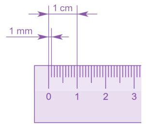
☐ In a ruler the 10 equal smallest parts are equal to one centimeter. One smallest part is equal to 1 mm.
